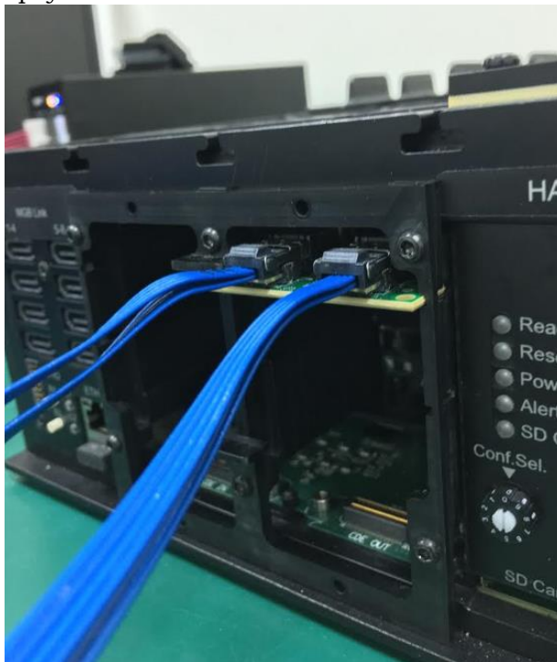
Figure 5: A FIREFLY_MGB Interface Card Installed on a HAPS-80
