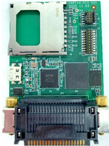
Figure 1: Top View of SDIO_EMMC5.1_HT3 daughter board
