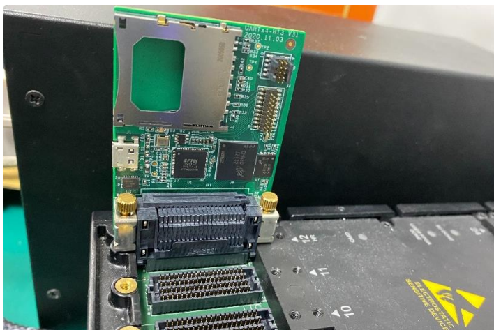
Figure 4: SDIO_EMMC5.1_HT3 mounted on HAPS-80 system
