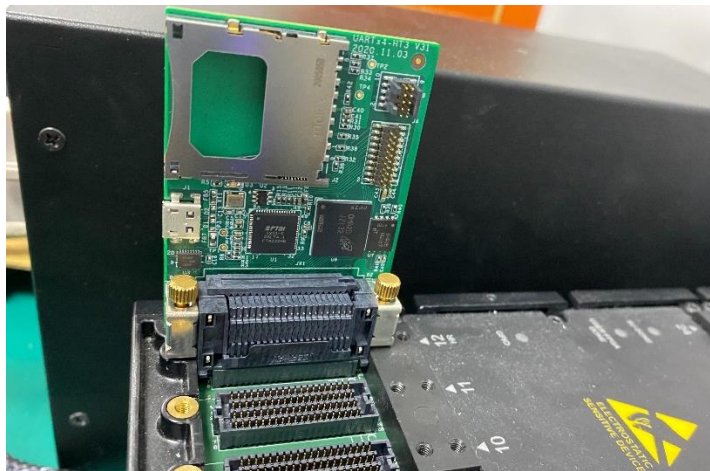
Figure 4: SDIO_EMMC5.1_HT3 mounted on HAPS-80 system
