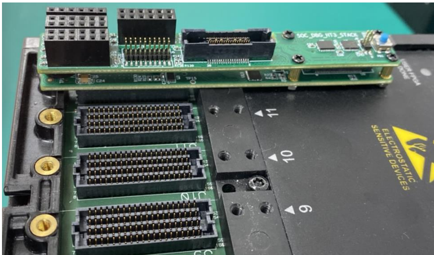
Figure 5: SOC_DBG_HT3 mounted on HAPS-80 system
