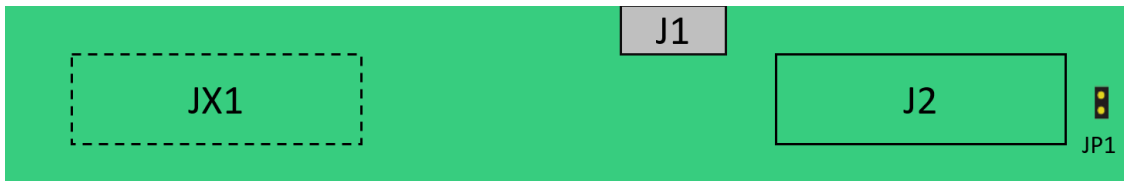
Figure 3: Top and Bottom(dotted line) of SOC_DBG_HT3 base board layout
