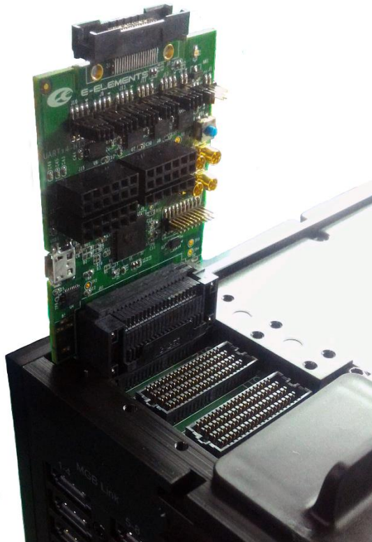
Figure 4: SOC_IOV_HT3 mounted on HAPS-80 system
