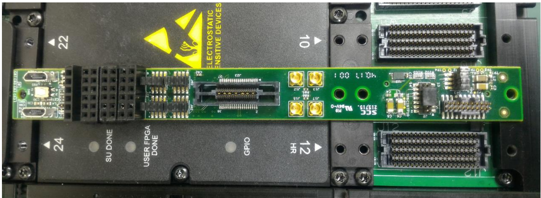
Figure 4: SOCIO_HT3 mounted on HAPS-80 system
