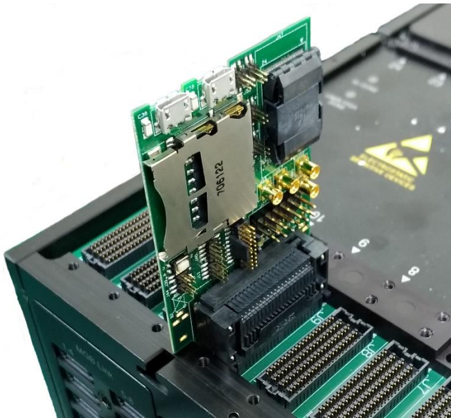
Figure 4: SOC_SDNF_HT3 installed on a HAPS-80
