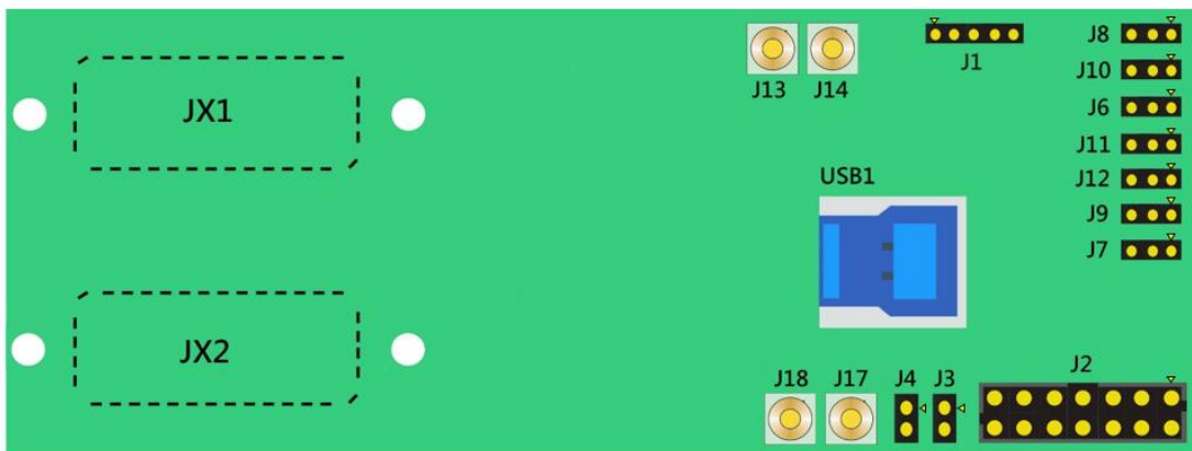
Figure 2: Top and Bottom(dotted line) USB3_HT3 Card Layout
